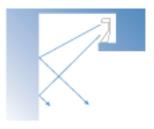
Wall washer using floating ceiling
