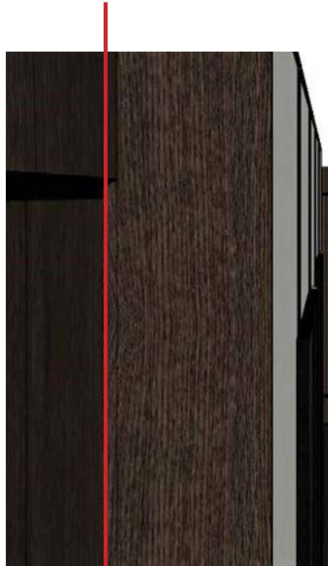
SIDES OF LARGE PANEL WALL RECESSED STRIP LIGHTING 3500K TEMPERATURE
