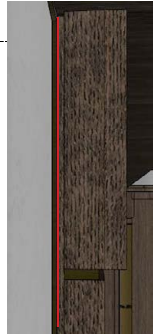
OTHER PANEL WALLS RECESSED STRIP LIGHTING 3500K TEMPERATURE
