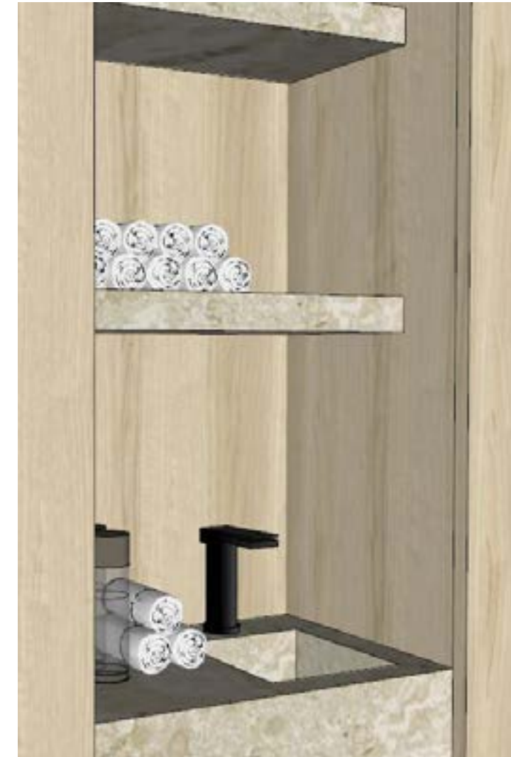
2500-3000K WALL WASH LINEAR LIGHT IN STONE COUNTER REVEAL. IN SHELVING, LINEAR LIGHT ON TOP AND BOTTOM OF SHELVING
