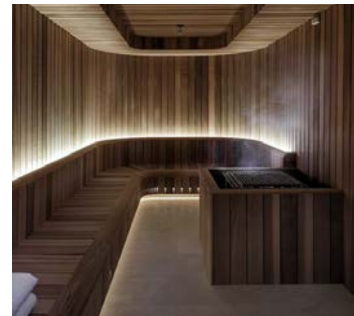
2500-3000K (DIMMABLE) IN SAUNA - CEILING AND BETWEEN WALL AND SEATING
