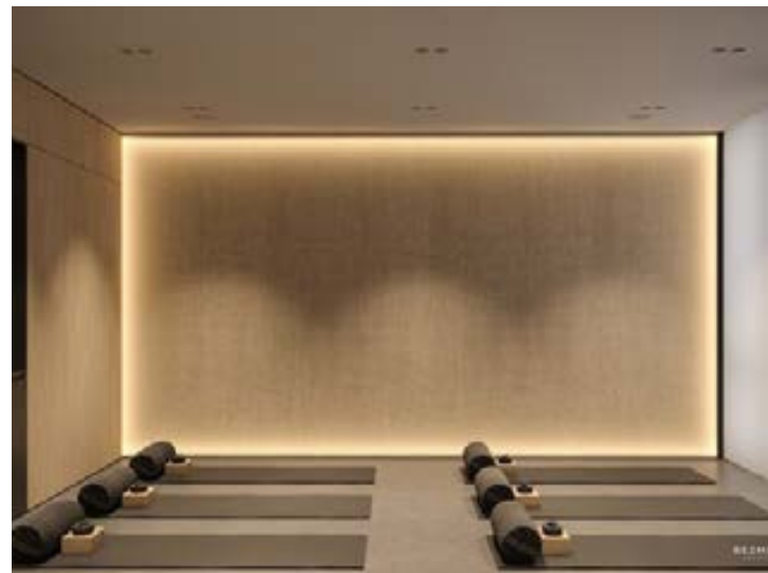
2500-3000K (DIMMABLE) WALL WASHED SPACE BEHIND YOGA "TEACHER" IN THIS AREA THERE ARE MIRRORS - DO NOT BACK LIGHT THESE
