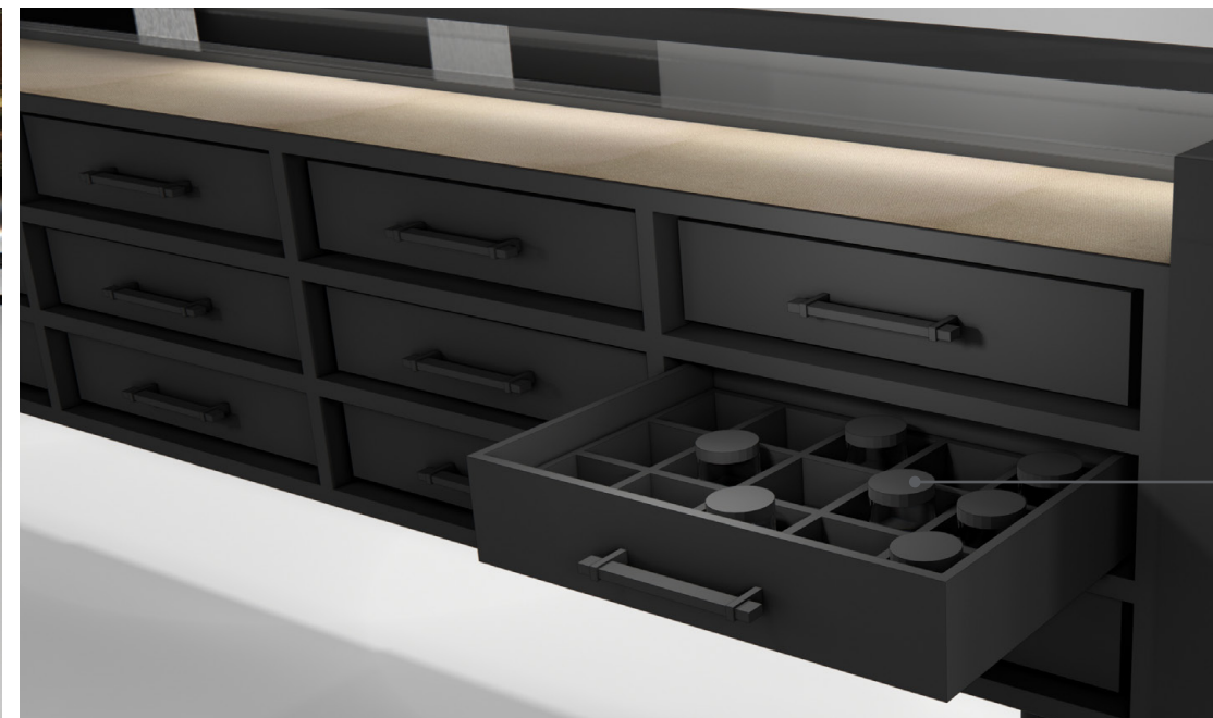
SENSORY EXPERIENCE BOXES IN CUBIES BEHIND BAR. TO HAVE SECURITY CABLE ATTACHED TO BACK OF CUBIE AS REQUIRED.
