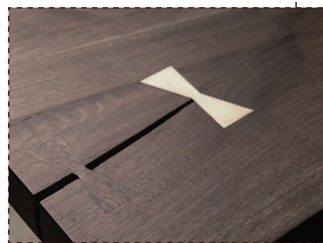
BUTTERFLY METAL JOINT ON SPLIT TABLE TOP 台面蝴蝶结式金属接头细节
