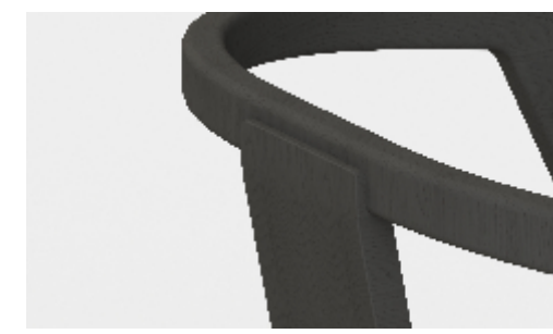
RENDERED VIEW OF JOINERY DETAIL WRAPPED LEATHER DYED TO MATCH LAQUER FINISH REFERENCE IMAGE B.
