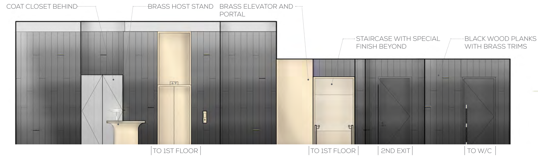
2 ELEVATION OF ELEVATOR NTS
