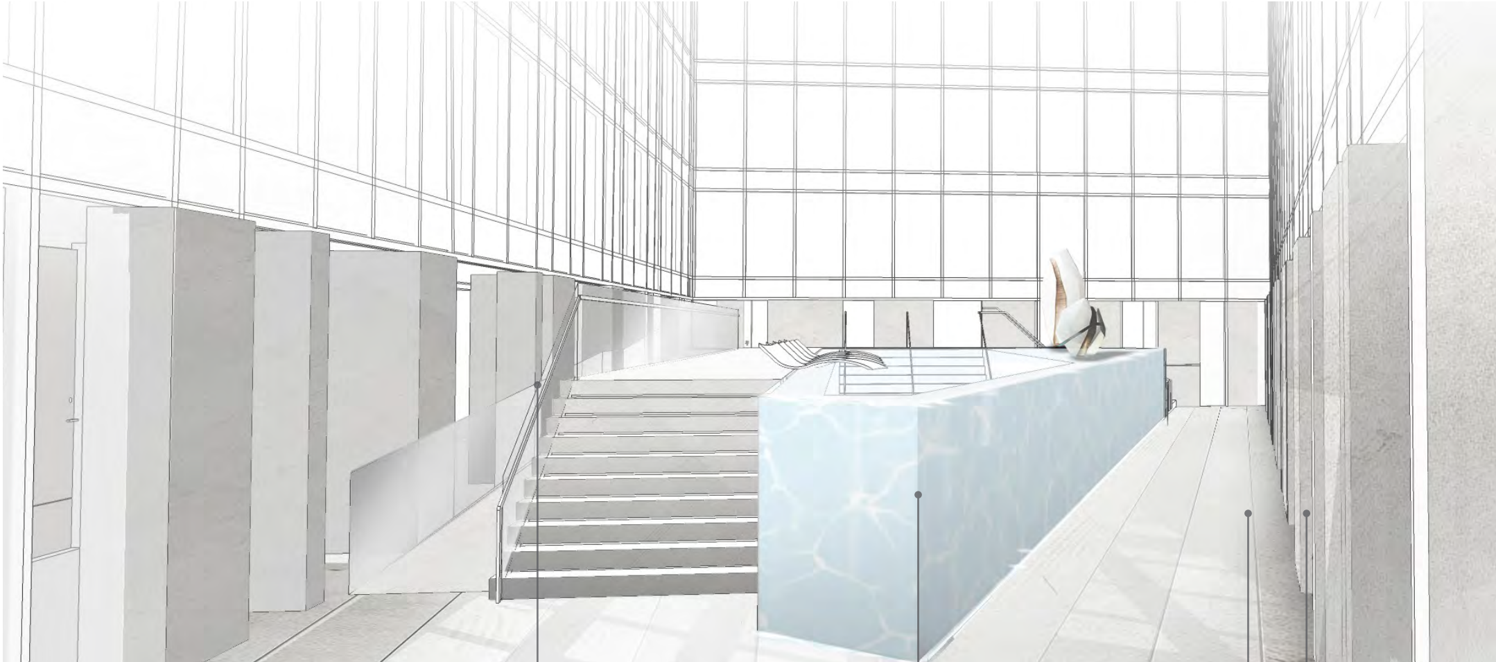
METAL RAIL WITH INTEGRATED GLASS GUARD
